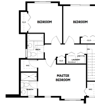
3 TYPE E1 - LEVEL 3 1/4" = 1'-0" FLOOR AREA = 70.03m 2 / 753.80 SF
